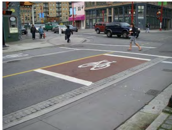
Bike box and cycle track, Carrall Street, Vancouver, BC
