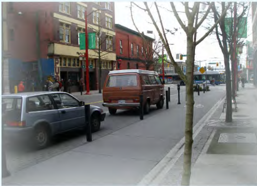
Cycle track separated from vehicle lanes by parking and boulevards on Carrall Street, Vancouver, BC. A cycle track is a protected bicycle route that is separated from vehicle traffic.
