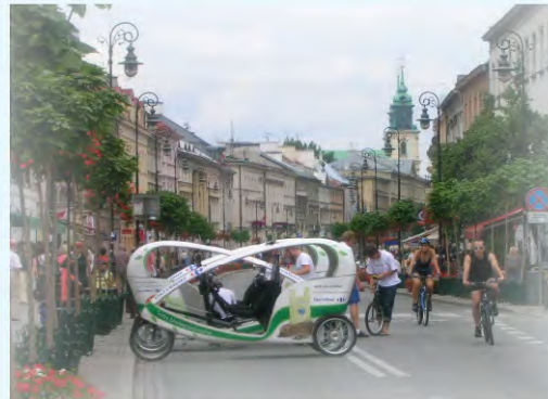
Pedicabs on car-free street in Poland. The pedicabs have fairings which improve aerodynamics and provide some protection from the elements.
