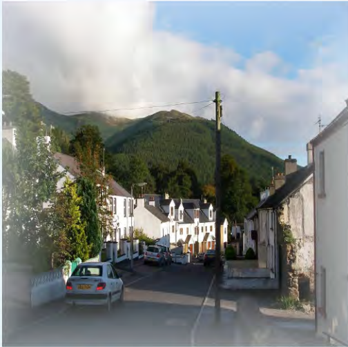
Local road in Northern Ireland. Narrow road encourages vehicles to move slowly.
