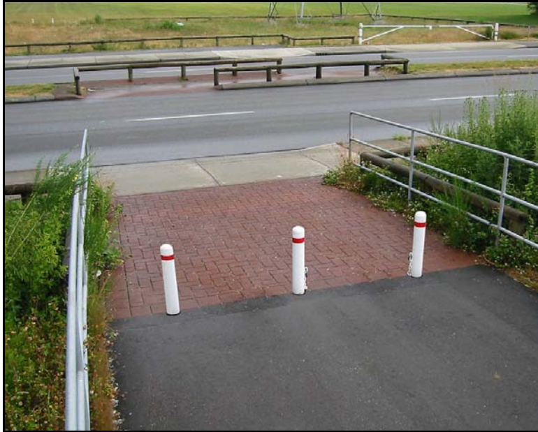
Figure 4.31 — Offset median island pathway crossing
