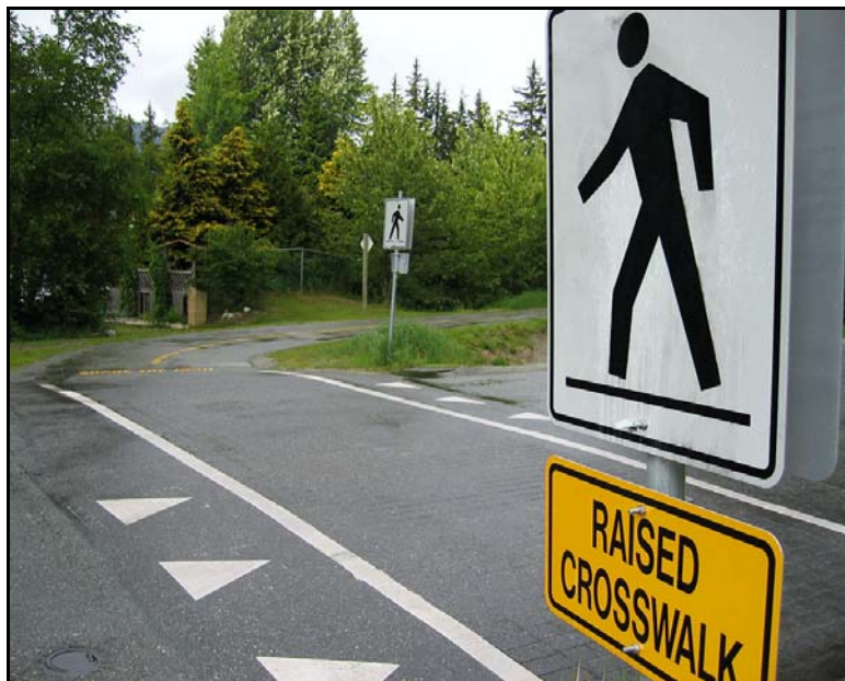
Figure 2.7 — Raised Pathway Crossing
