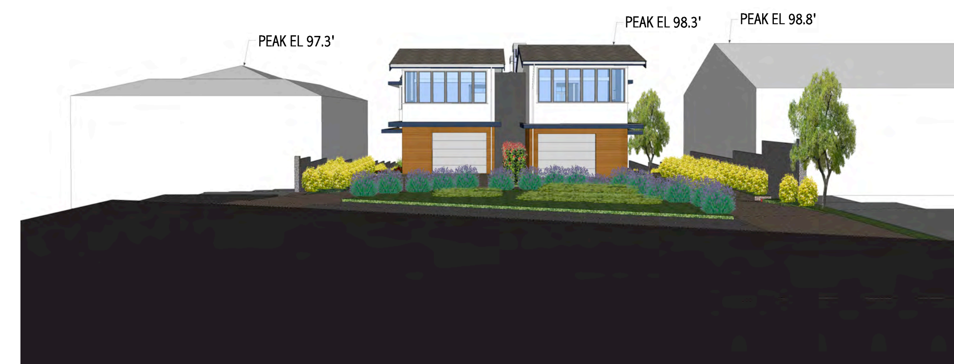
RELATIVE ROOF PEAK ELEVATIONS
