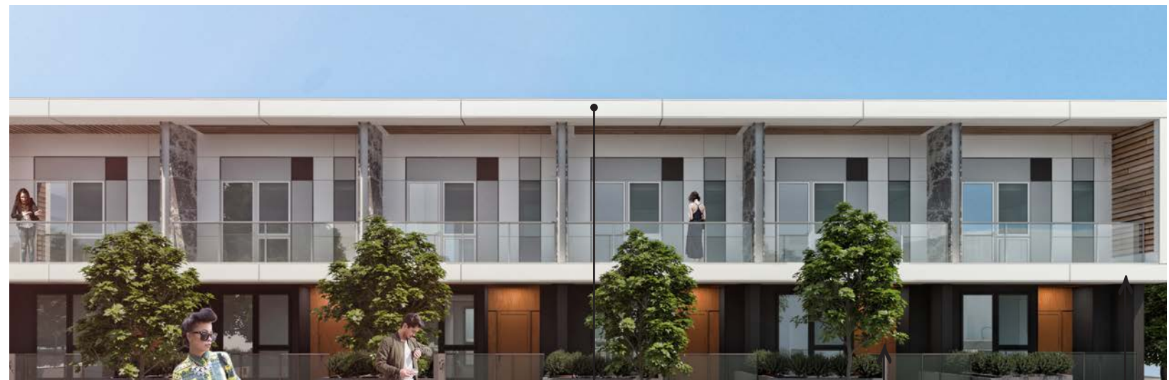
Extruded overhangs provide passive solar control
