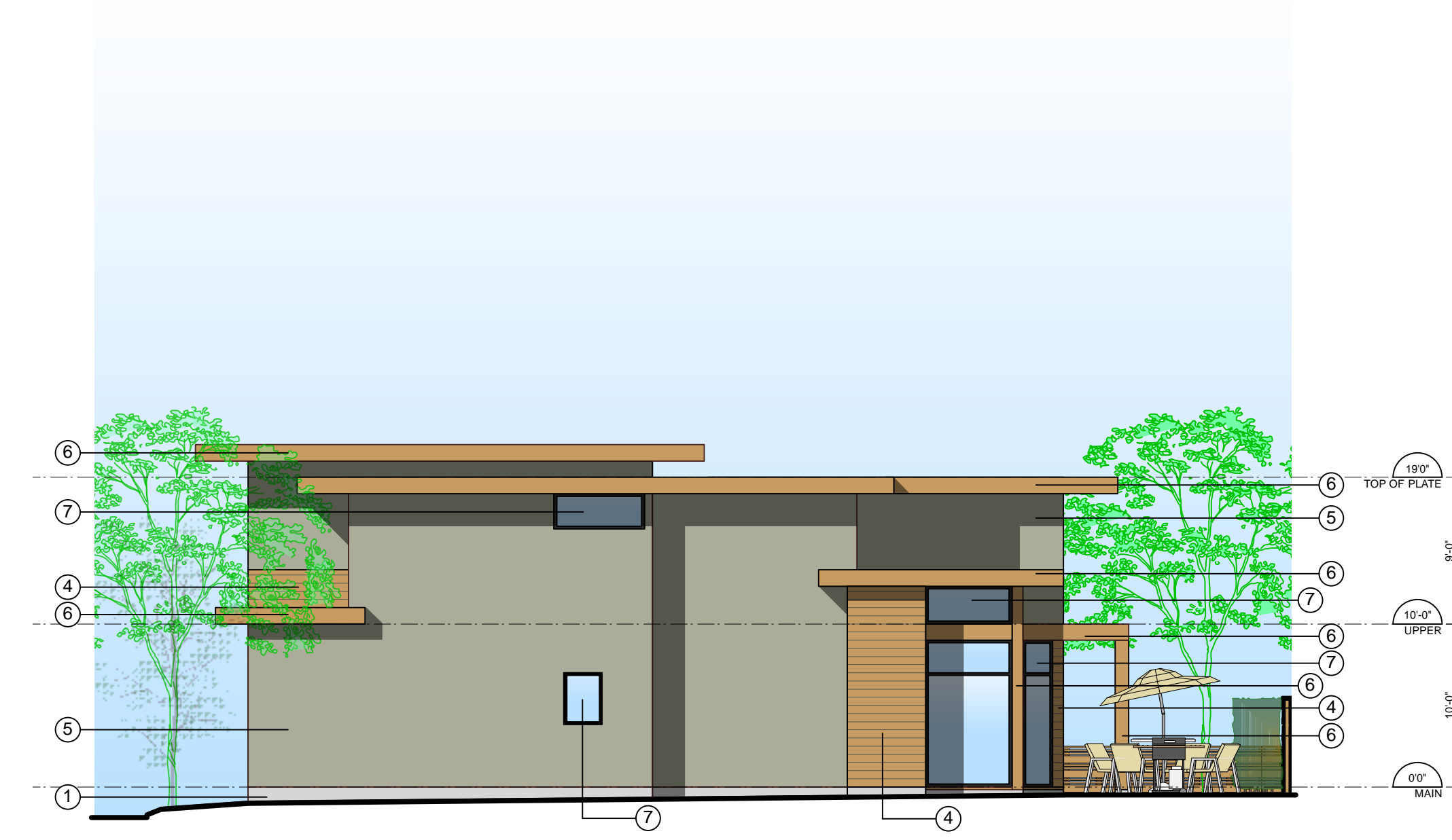
2 North (Side) Elevation - Buildings 2, 4 & 6 1/8" = 1'-0"
