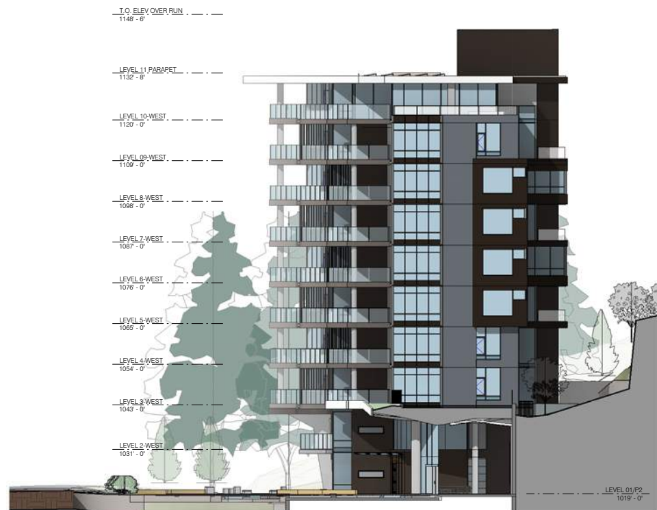
2 Tower East Elevation 1/16" = 1'-0"
