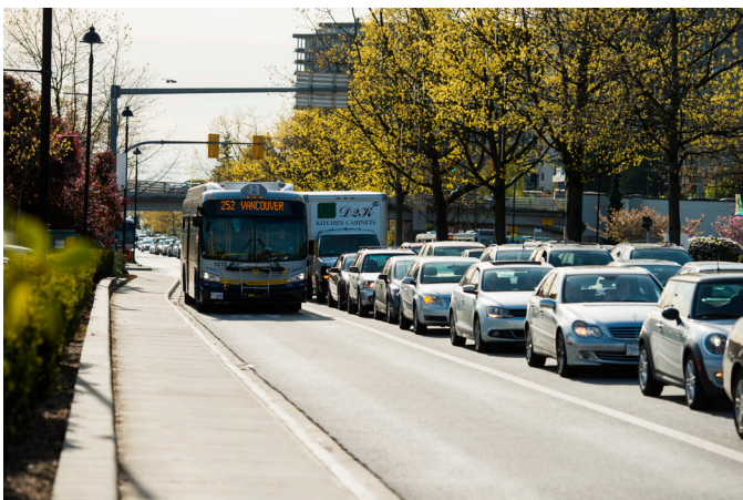
Figure 2.4 - Public Transit: Example of queue jump bus lane
