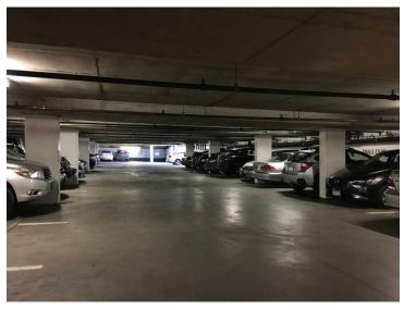
stockpiles of combustibles do not exceed 8 feet (2.4 m) and fires with moderate rates of heat release are expected. Other examples of Ordinary Hazard Group 1 are restaurant service areas, automobile showrooms, and bakeries.
