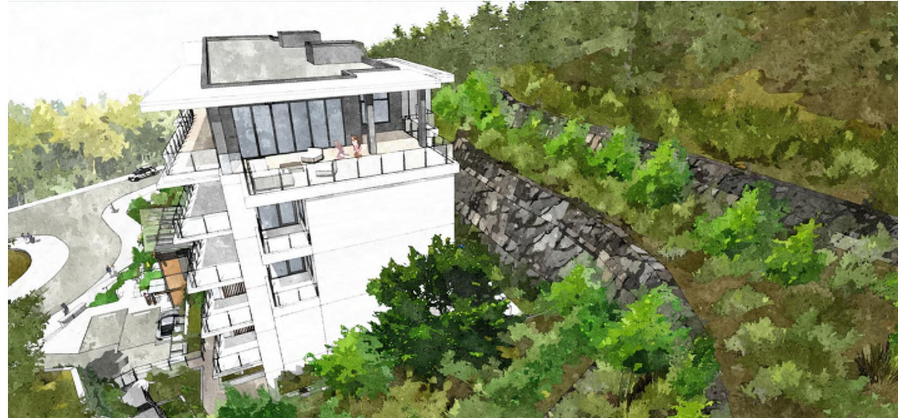
Overall, the planting design follows the FireSmart guidelines, including plant selection, the locating of trees at least 3m from the building, and use of non-flammable hardscape materials within 1.5m of the building.
