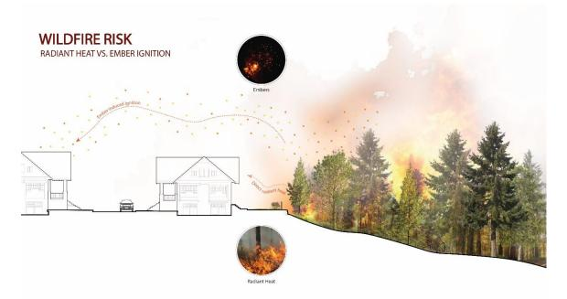
Figure 6. Ignition pathways in the interface. Radiant heat threatens structures within 10m of the forest edge while embers spread to structures within the interior of the development.
