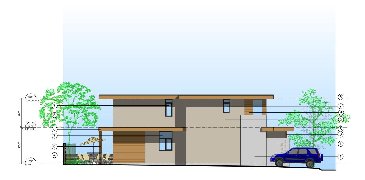
4 South (Side) Elevation - Buildings 3 & 5 North (Side) Elevation - Mirrored for Building 7 1/8" = 1'-0"
