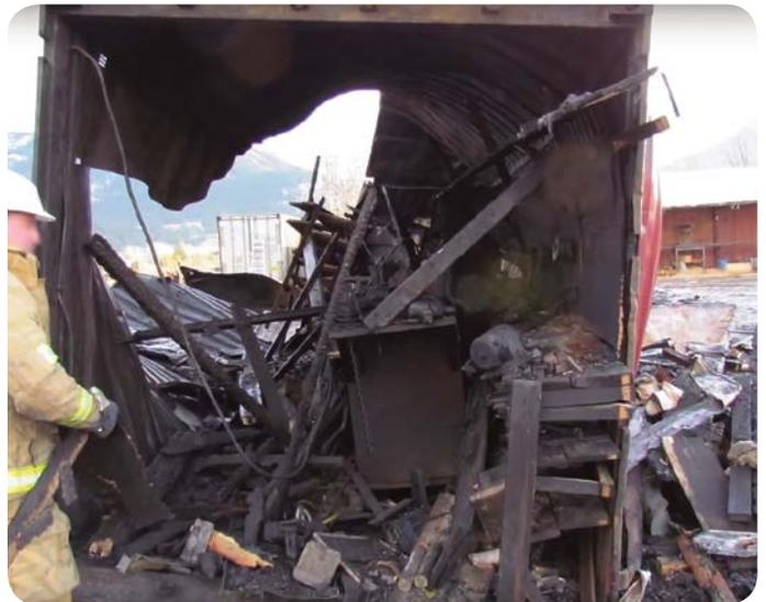
explosion during a fire response at a building next to the container. In another incident, a propane leak from a barbecue stored inside a shipping container caused an explosion that blew one of the 113-kilogram doors 40 metres away.
