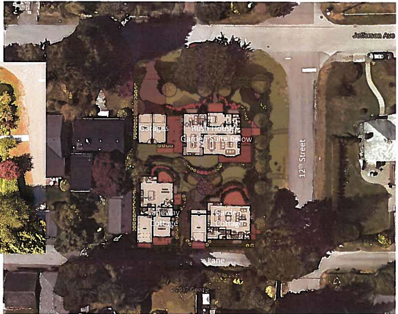
Site plan showing the relocated Rush House, and new infill cottages. The front setback for Rush House along Jefferson Avenue remains the same as present. The setback along 12 th Street matches that of the houses along the north side of Jefferson Avenue and south across the lane.
