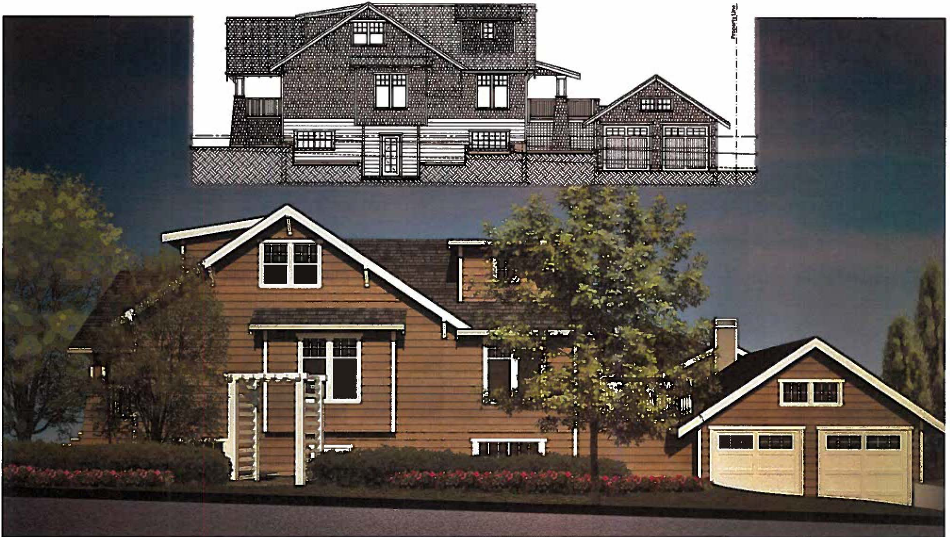
Earlier elevation showing Rush House and the new garage structure. A dormer has been added, as suggested by the architect and heritage consultant, to give Rush House a more impressive appearance from the street.
