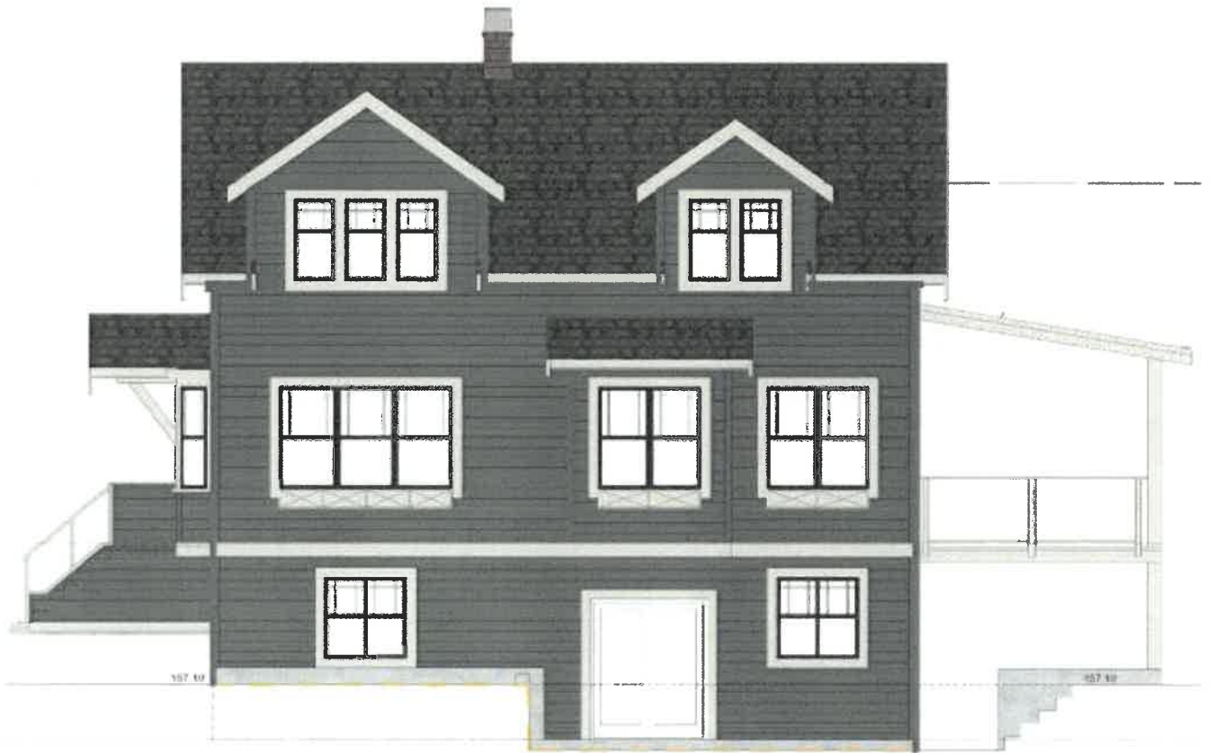
Figure 76: Proposed south elevation with new dormer and basement entrance _ Focus Architectural Inc
