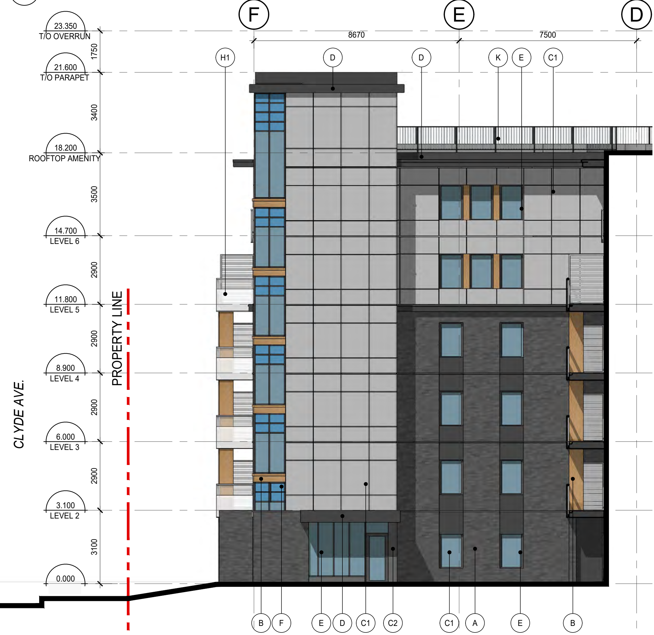
2 EAST ELEVATION - COURTYARD 1:100
