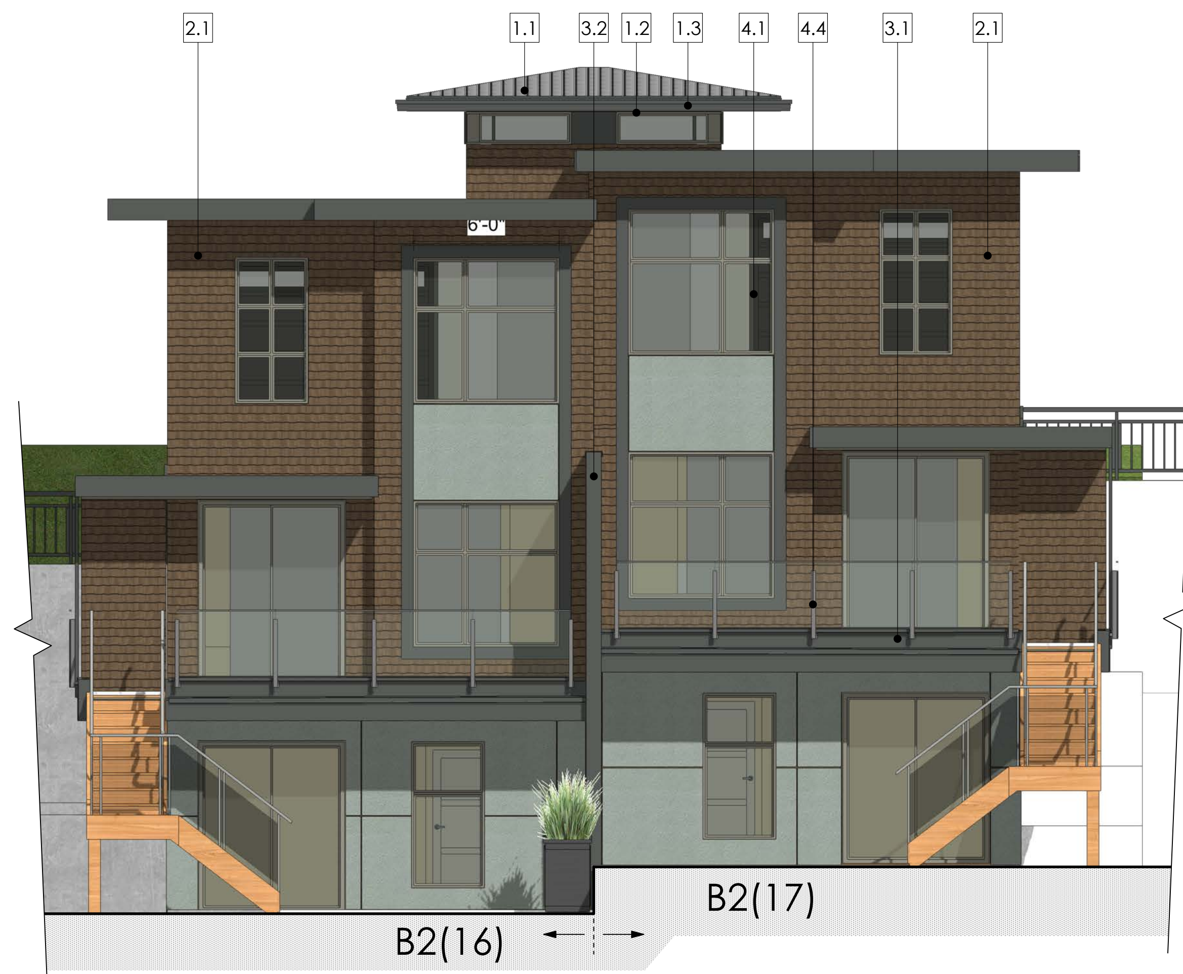
BACK ELEVATION UNIT B2
